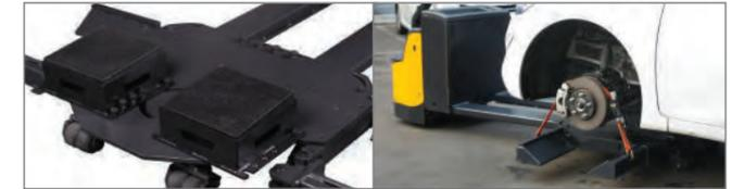
9 Moving of wheelless automobile Cross member supports automobile
