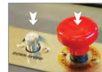
Table down speed control valve & Main circuit cutoff switch
